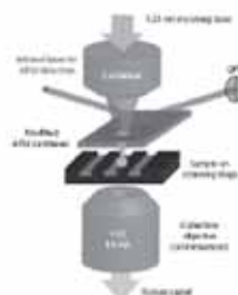
Figure 2. Sketch of the experimental set-up, showing the integration of the photonic-plasmonic device into an AFM-Raman microscope
